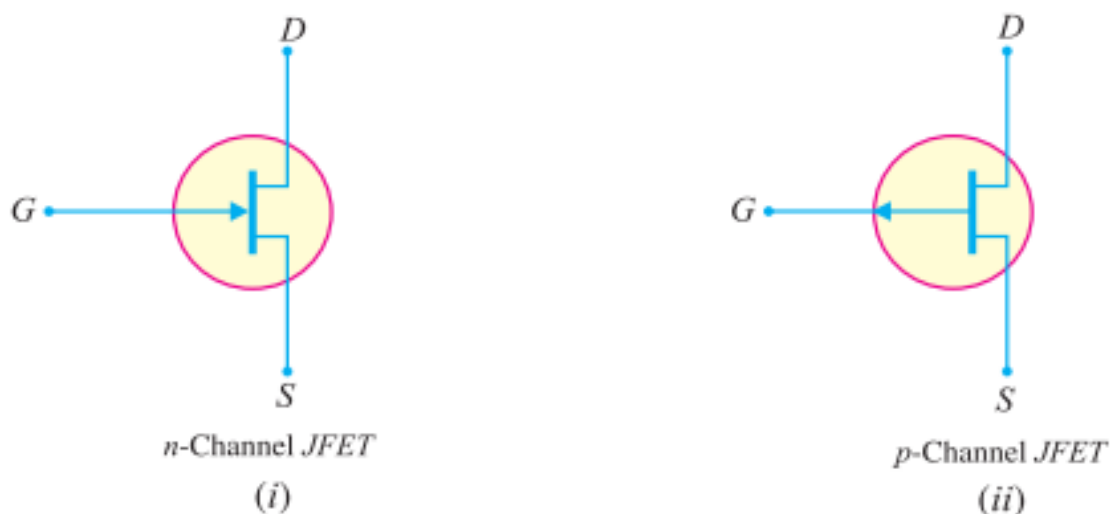
Figure 2.6 Schematic Symbol of JFET
